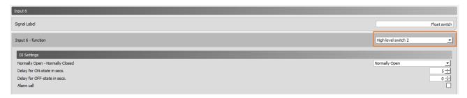
3. In addition, there are 2 other registers to be set. To access these, select the function menu "Graphic View / Schematic View". The two registers to be changed are "time" for unchanged level measurement, and "Hysteresis" for unchanged level measurement.
