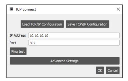
Enter the IP address and port to get remote control of SPIDER via TCP / IP. Upon contact, the program located in the SPIDER is retrieved. It is then possible to either make changes online in the SPIDER or save a copy of the current program locally and then work on it.
