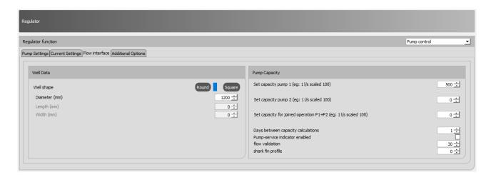
With very few settings, SPIDER can perform a validated flow calculation. You choose whether the shape of the well is round or square, then enter either diameter or the dimension of the sides in mm. This determines the surface area and SPIDER calculates on the basis of the start/stop levels how much is pumped out during a pumping cycle.
