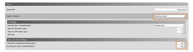
2. To access the "High level switch 2 function", the function selection "High level switch "must be changed to "High level switch 2".
