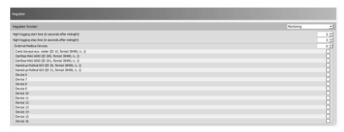
The SPIDER control can be used as a pure monitoring device and by selecting this feature, SPIDER no longer acts as pump control. It will now use ModBus communication to the selected device type installed.
