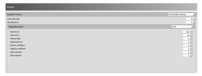
By choosing ground water level the SPIDER can keep a constant water table level. Sensor elevation is the top of the sensor tube in relation to a given terrain point. In Denmark it is called "Kote DVR90". The sounding
