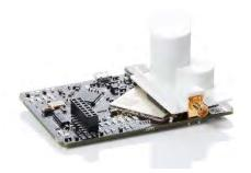
SPIDER is equipped with a built-in Power bank and can send voltage failure alarms when the primary power supply disappears.
