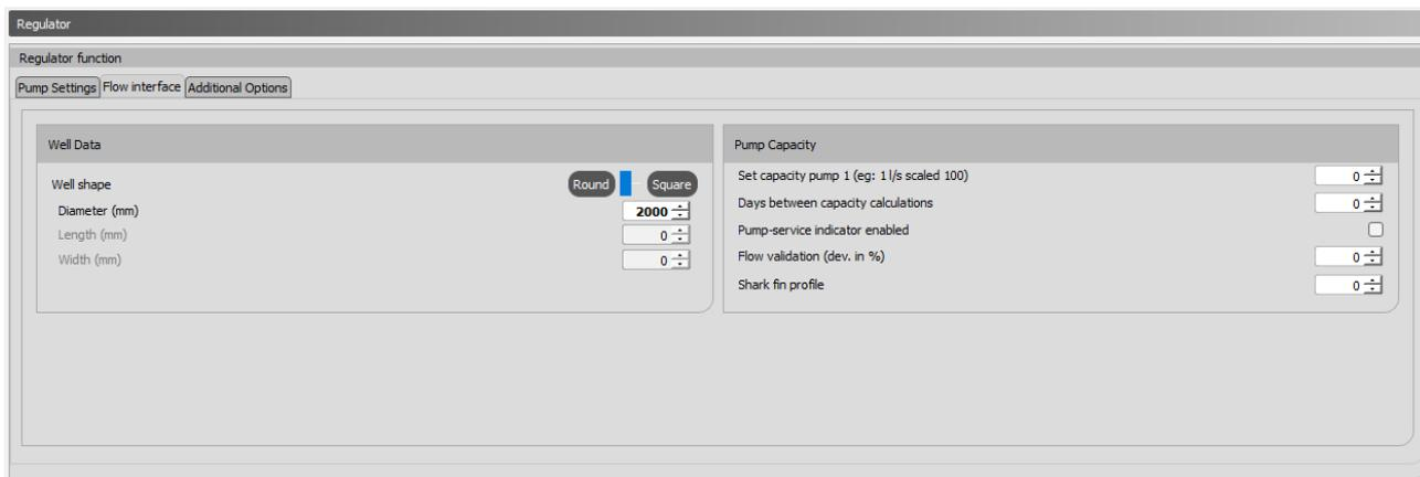
When specifying the physical design of the well, the PUMA controller subsequently calculates the following data, which are available via the SCADA-system. It is therefore possible to get a load and performance profile of the pumping stations, without having to invest in external measuring equipment for the individual stations.
