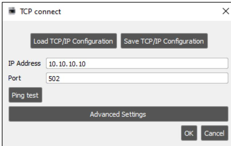
Enter the IP address and port to get remote control of PUMA via TCP/IP. Upon contact, the program located in the PUMA is retrieved. It is then possible to either make changes online in the PUMA or save a copy of the current program locally and then work on it.
