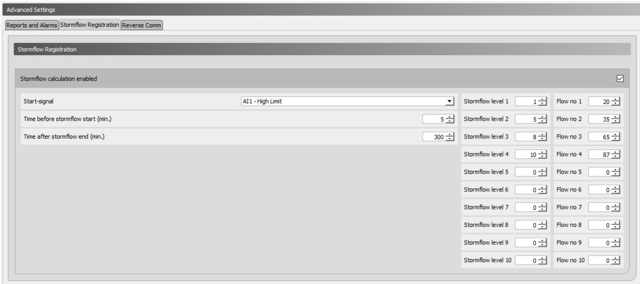
Stormflow calculation is used to record the number, duration and quantity of stormflow events.
