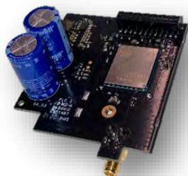
PUMA's communication module is equipped with a built-in power bank and can send voltage failure alarms if the primary power supply stops working.
