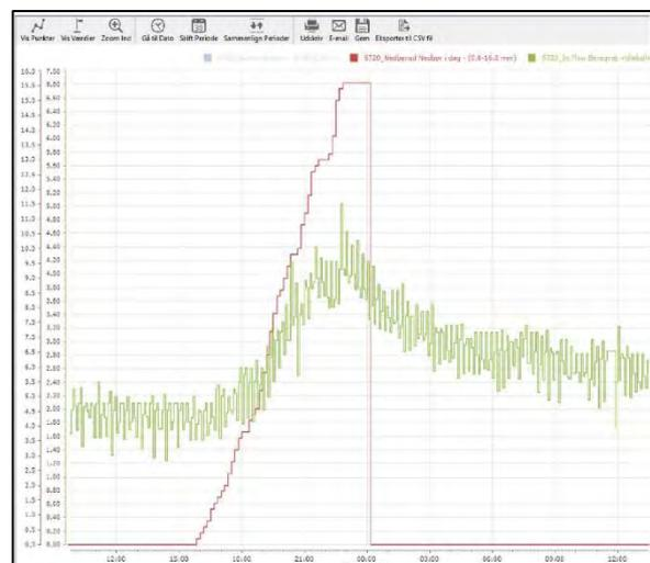
e.g. 3-4 hours before the increased inlet flow, there would be an indirect inflow, which in most cases is due to drains or seepage of groundwater into the system.
