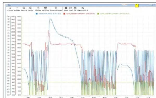
The image is an example of a curve showing the current level (blue), outlet flow (green) and inlet flow (red).
