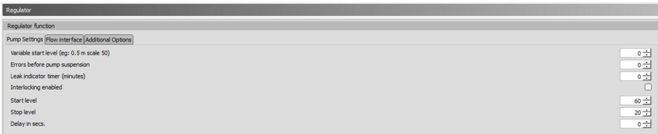
Under the settings for AI1 is the regulator function. Here, the most common parameters for the pump control function are configured.
