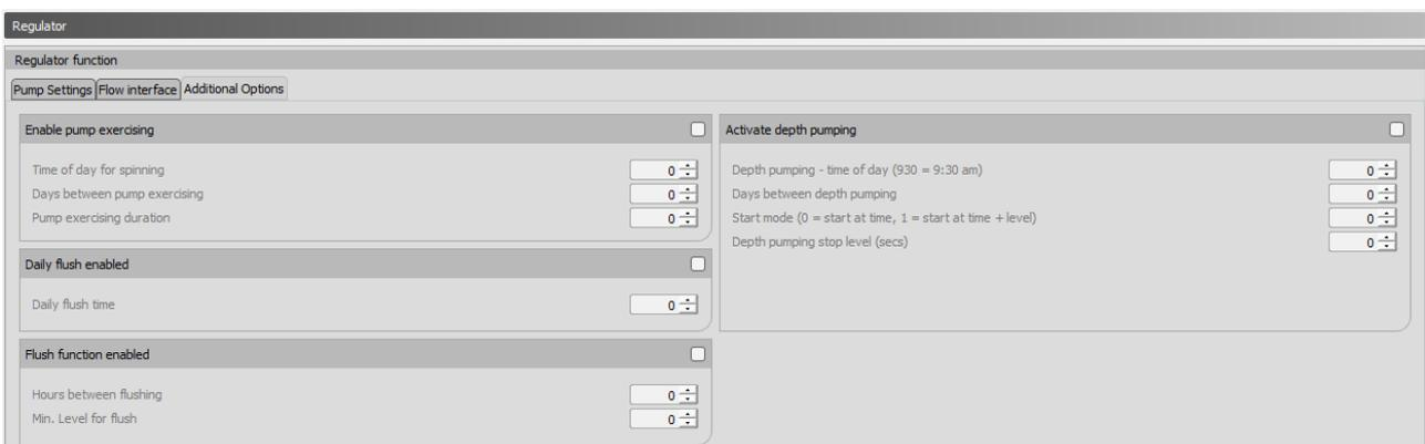
It is possible to select 4 different maintenance functions. The functions are activated by ticking the individual functions.
